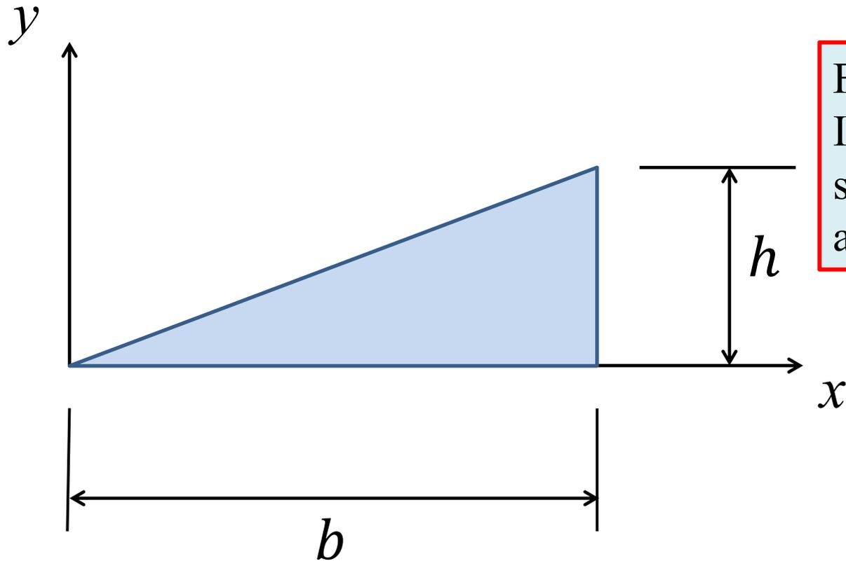
Find the Moment of Inertia of the shaded area about the  $x$  and  $y$  axes shown.
