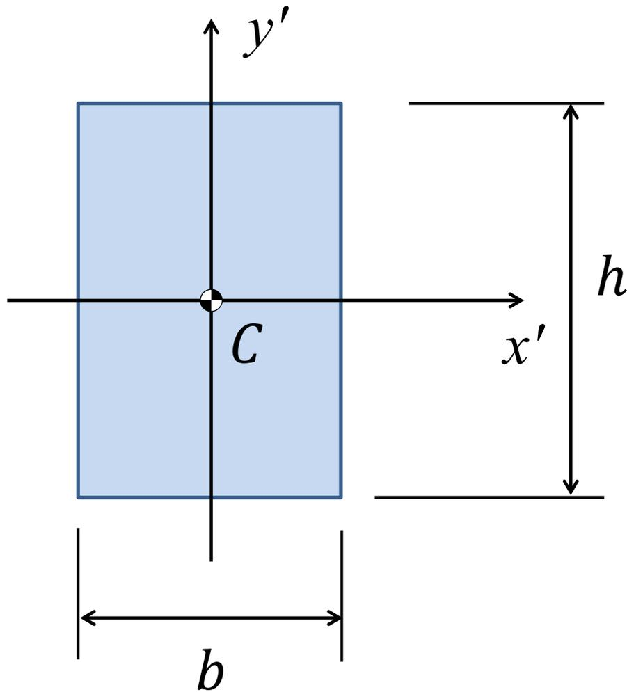
Find the Moment of Inertia of the shaded area about the centroidal  $x'$  axis
