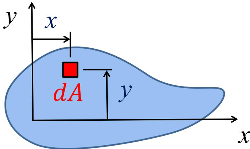
Recall we used the first moment of the area about an axis to find the centroid. The **Moment of Inertia** is the second moment of the area about an axis
